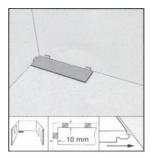
The installation begins at the left hand side of the room, with the 2 tongue edges of the laminate board facing the walls, an expansion gap will need to be left with a minimum of 10mm.
