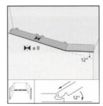
The second plank is connected into the groove on the short end of the already laid plank at a slight angle and then lowered to the floor, the row is built up in this manor, the final board will need to be cut observing the 10mm expansion.
